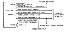
Figure 7. Example: Command Register = 00111001
